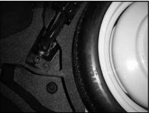
STEP 5 Position the spare tire and Stealthbox® so the spare tire matches up with the curve of the left side foam panel.
